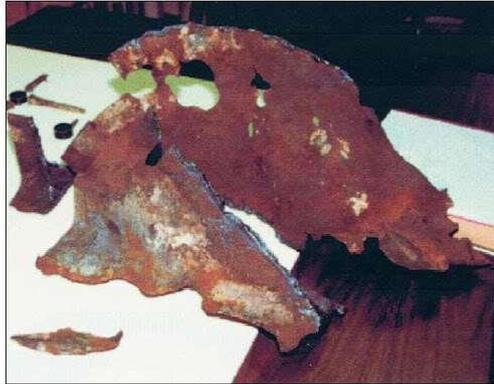
Figure C-1 Eroded A36 wide-flange beam.
