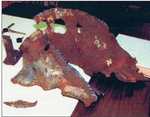
Figure C-1 Eroded A36 wide-flange beam.
